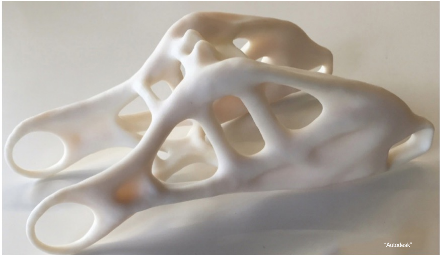
Motorcycle swingarm: the piece that hinges the rear wheel to the bike's frame
